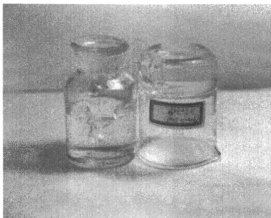
Figure 3. Typical nearly transparent PMMA hydrogels. (Reproduced from reference 5. Copyright 1999 American Chemical Society.)
