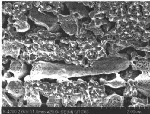
Figure 11. Cryo-fractured SEM image of a Gluconobacter oxydans coating (52, 57). A. Top coat surface showing fissures. Cryo-fracture of top coat showing fissures and polymer particle pull-outs. C. Cell coat showing pore space surrounding latex-embedded and cryo-fractured G. oxydans.
